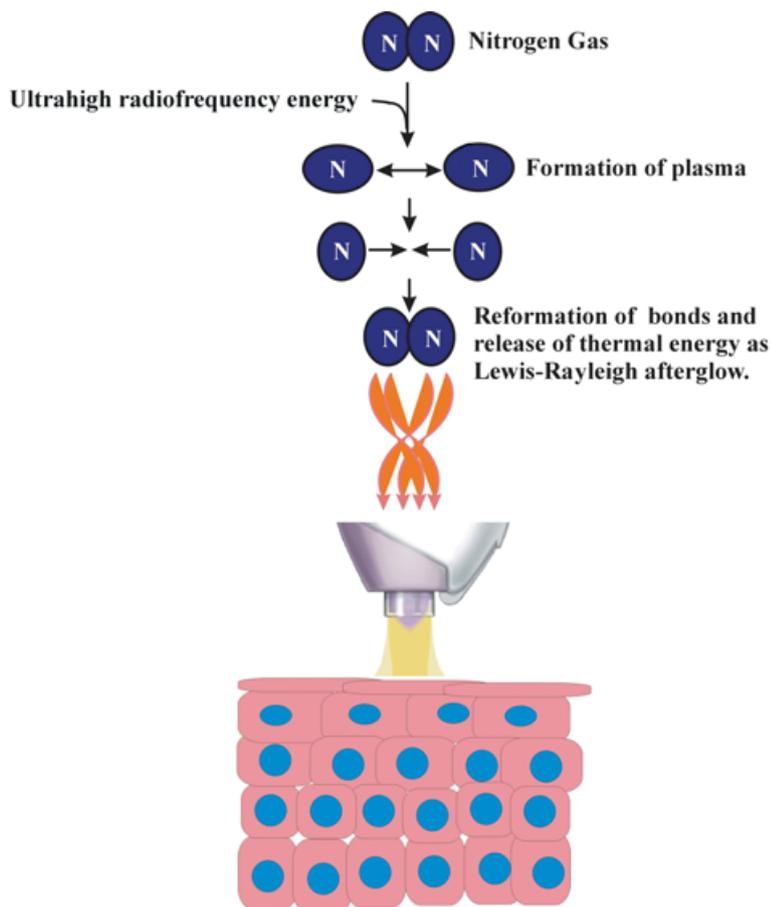
**Figure 1** Plasma generation. An ultrahigh frequency radiofrequency generator excites a tuned resonator and imparts energy to nitrogen gas molecules flowing through the handpiece resulting in their ionization. The plasma is directed through a quartz nozzle out of the tip of the handpiece and onto the skin, and appears as a characteristic lilac glow that transitions to a yellowish light called a Lewis–Rayleigh afterglow.
